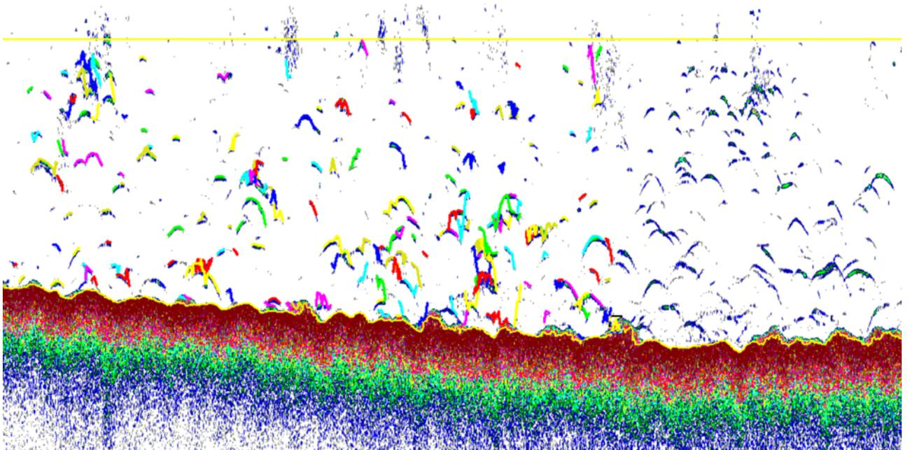
**Figure 5.** Biomass estimation using Sonar5 Pro for a BR transect, showing individual detected “fishes” (multicoloured arches).
