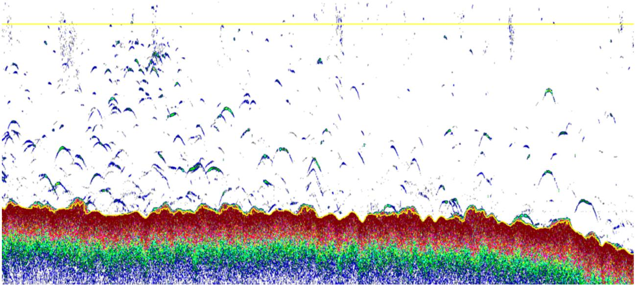
Footnote: Bottom yellow line is the algorithm-detected seabed using the thresholding parameters and the top yellow line demarcates the 2 m depth mark. The water column between yellow lines defines the analysis window.
